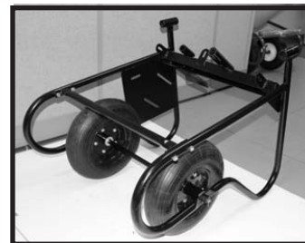
Fig.7: Correctly set-up frame assembly.
