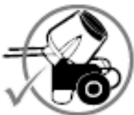
Fig.41: Correct placement of handles for WORKING position.
