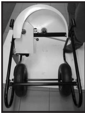
Fig.38: Remove mixer drum and place drum gear guard over mixing drum gear. This guard wraps over the drive assembly guard.
