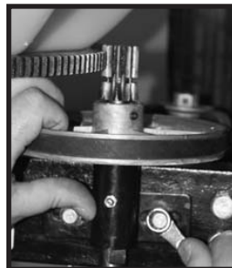
Fig.25: Centre mixing drum gear onto drive gear and tighten jackshaft plate to set adjustment.
