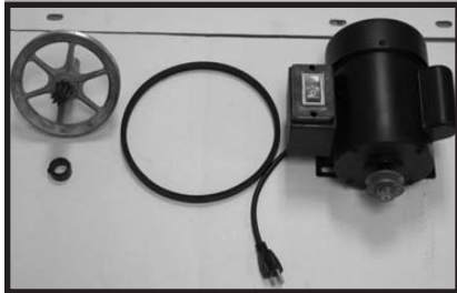
Fig.14: Parts required for mounting motor and drive assembly.
