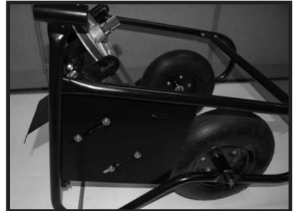
Fig.29: Frame assembly with drive belt, drive assembly and motor
