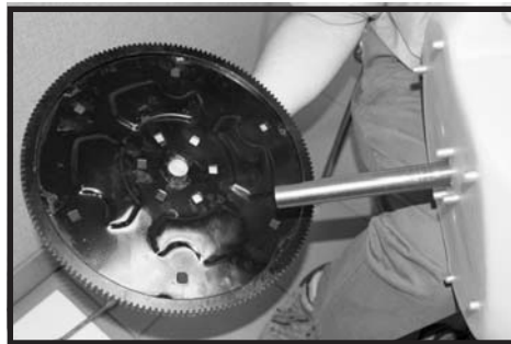
Fig.12: With drum on its side, slip mixing gear onto drum shaft and add nuts to secure assembly.
