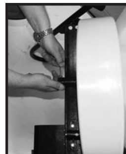
Fig.40: Replace and tighten lock rings on jackshaft and mixing drum shaft.
