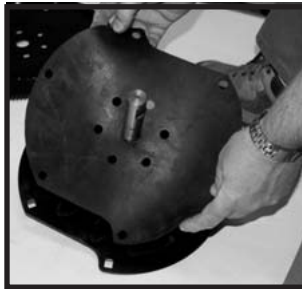
Fig.9: Line up holes on both rubber pad and plate assembly.
