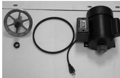
Electric motor, drive belt, jack-shaft and lock ring.
