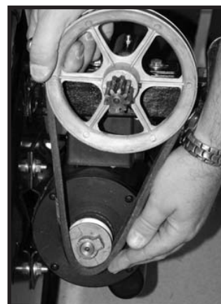
Fig.20: Slip drive belt onto pulleys.
