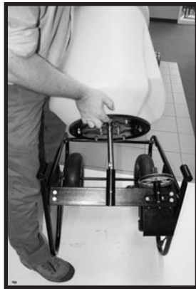
Fig.31: Place mixer drum onto drum support mount.
