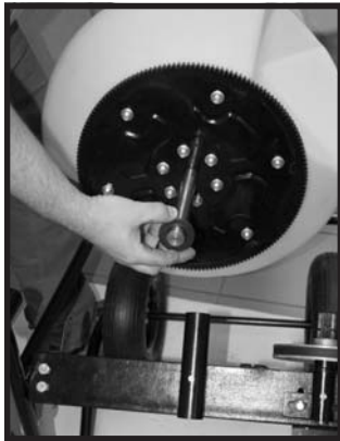
Fig.30: Slide washer onto mixer drum shaft.
