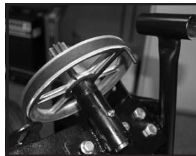
Fig.18: Incorrect positioning of lock ring for jack shaft.
