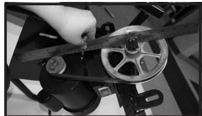
Fig.26: Verify adjustments with ruler.
