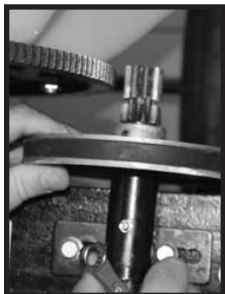
Fig.24: Loosen bolts on jackshaft adjustment plate to shift drive assembly.
