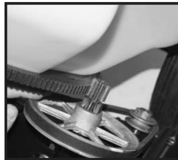
Fig.33: Turn mixing drum to check for smooth operation of mixer. Make sure drive gear and mixing gear are centered and flush to each other.
