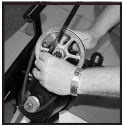
Fig.21: Use a ruler as a guide to belt adjustment.
