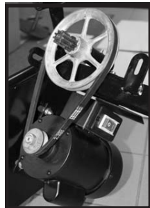
Fig.28: Correctly mounted drive belt, drive assembly and motor
