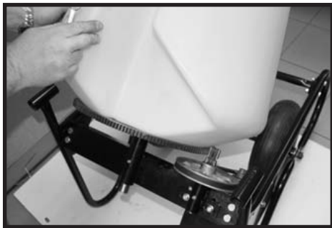
Fig.30: Slide washer onto mixer drum shaft.
