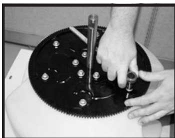
Fig.11: Slide bolts through drum attachment assembly and mixing drum by turning the drum onto its side.
