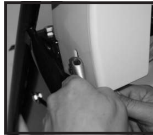
Fig.39: Bolt guards to frame. Note placement of drive gear for clearance from guard. Tighten as shown.
