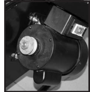
Fig.16: Align motor to mounting slots on left frame and bolt in place.
