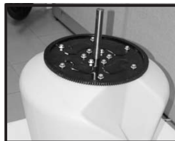
Fig.13: Turn drum assembly over and complete tightening of bolts.
