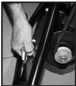
Fig.27: Loosen motor mounting bolts to move motor for further adjustments as needed.
