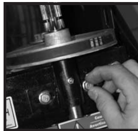
Fig.22: Finger tighten bolts on adjustment plate for a rough setting of belt adjustment.
