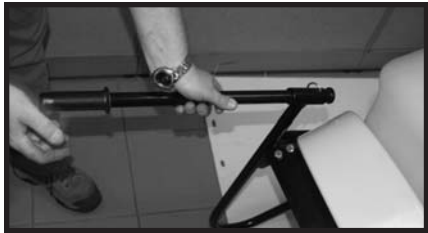
Fig.41: How to install handles.
