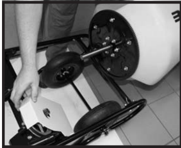
Fig.35: Remove mixer drum and place plastic motor guard over drive mechanism.
